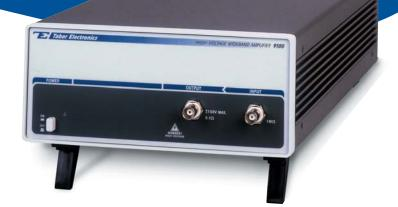
Model 9100 is a Single-Channel, 2U, half-rack size, bench-top power amplifier designed for signal amplification. With unprecedented signal purity, Model 9100 amplifies signals from dc to over 500KHz. The unit has a fixed gain of x15 however the same amplifier is available with custom gain and no signal purity or performance degradation whatsoever.
